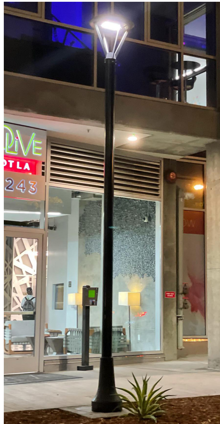
Street lighting fixture approved by Bureau of Street Lighting for use on Melrose: 14' AV Steel Pole with Cree edge round luminaire (spider)
